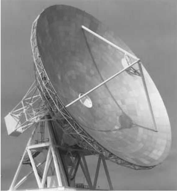
Figure 8.7 Standard-A (C-band 6/4 GHz) 32-m antenna. (Courtesy of TIW Systems, Inc., Sunnydale, CA.)
